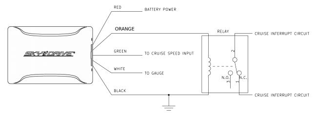
AS A SAFETY FEATURE, THE SKY DRIVE IS DESIGNED TO TURN OFF THE VEHICLE'S CRUISE CONTROL IN THE EYENT OF A LOST GPS SIGNAL. A TWO-SECOND, 12-VOLT PULSE IS PROVIDED ON THE BROWN WIRE TO DRIVE A RELAY COIL, WHICH MUST BE WIRED INTO THE VEHICLE'S CRUISE CONTROL INTERRUPT CIRCUIT.
