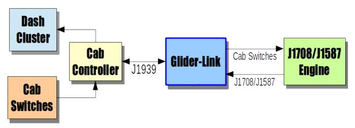
Cab switches include clutch, parking/service brake, retarder, cruise control, and fan override switches.
